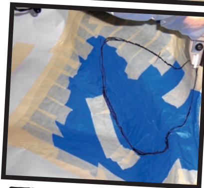
STEP2: Make an outline of the kickpanel on the tape with a black marker.
