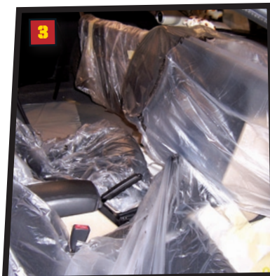
STEP1: Begin by taping up the driver and passenger side floor. Put about 2 layers and make sure that you keep the tape as flat as possible.
