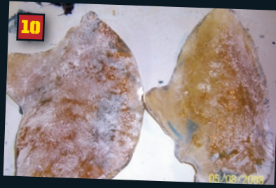
STEP10: Now you should have the bottom mold of the kickpanel that looks a little unfinished. However since you outlined your shape with a marker before you should now have an outline in your mold. Taking a jig-saw cut out along that line to give you a finished mold. Or if you find that using the jig-saw is too hard and have a dremel available put on the sand tool sand down/along the line till you have a finished mold as I did.
