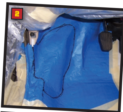
STEP1: Begin by taping up the driver and passenger side floor. Put about 2 layers and make sure that you keep the tape as flat as possible.
