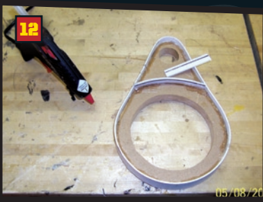
STEP12: Now taking those tracing the speakers trim ring again but this time the inside of it. Cut out these holes and check for speaker fitment. Cut more as necessary or sand if it is just a little tight. Now if you want to make the speakers flush mounted in the kickpanel grab some 1/4-inch ABS plastic and cut some 3/4-inch strips. Taking a hot glue gun, glue the strip flush to the edge of the ring around the outside. You can also add little pieces on the inside to separate the mid and tweeter as well as add a little more of a look as I did.
