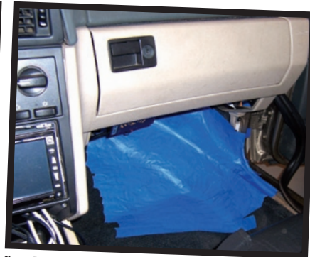
STEP1: Begin by taping up the driver and passenger side floor. Put about 2 layers and make sure that you keep the tape as flat as possible.
