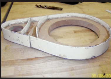
STEP12: Now taking those tracing the speakers trim ring again but this time the inside of it. Cut out these holes and check for speaker fitment. Cut more as necessary or sand if it is just a little tight. Now if you want to make the speakers flush mounted in the kickpanel grab some 1/4-inch ABS plastic and cut some 3/4-inch strips. Taking a hot glue gun, glue the strip flush to the edge of the ring around the outside. You can also add little pieces on the inside to separate the mid and tweeter as well as add a little more of a look as I did.
