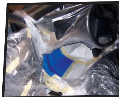
STEP3: Make sure to cover your seats, dashboard and any other parts of your interior that you want to protect from stray resin.
