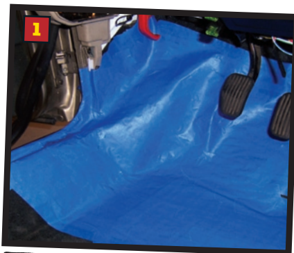
STEP1: Begin by taping up the driver and passenger side floor. Put about 2 layers and make sure that you keep the tape as flat as possible.
